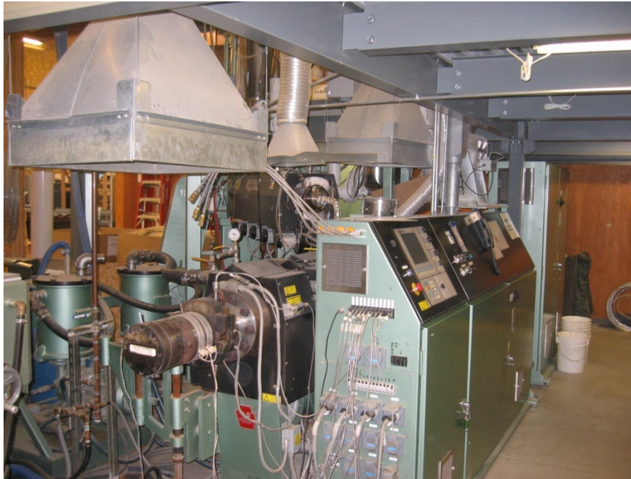
Figure 1 : Davis-Standard WT94 Twin Screw Extruder. To produce WPC boards about 14 cm (wide) and 4 cm (thick). Rate of production: 4 feet/min
