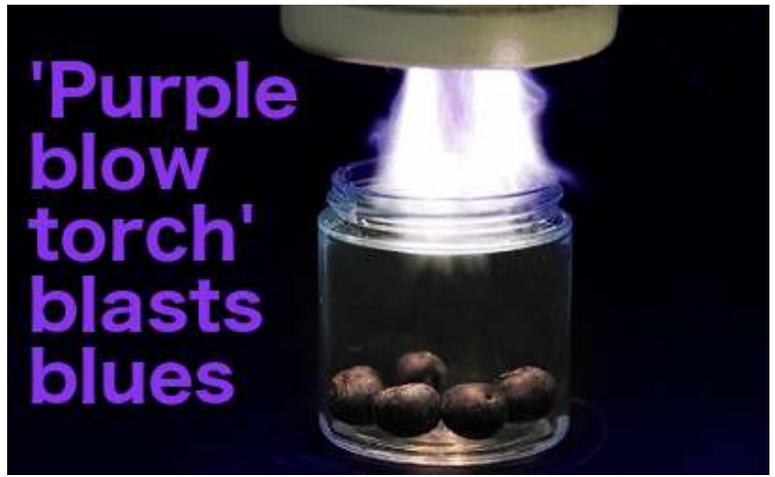
**Figure 1** Photo of Atmospheric Plasma flame treating a sample of blueberries. (From ref. 2)
