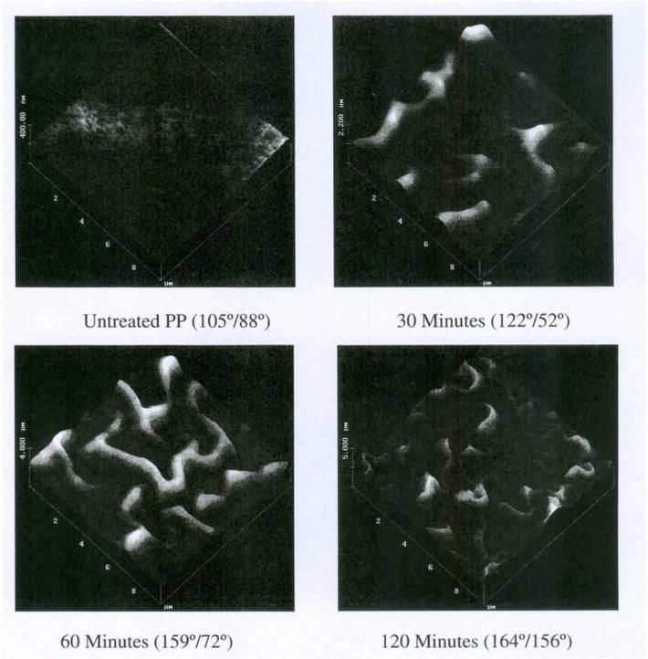
**Figure 2** AFM micrographs showing the increase in roughness of a poly(propylene) surface with increased exposure to an argon ion plasma. The numbers in parentheses are the advancing and receding contact angles of the respective surfaces. (Adapted from figure 9 of ref. 3)
