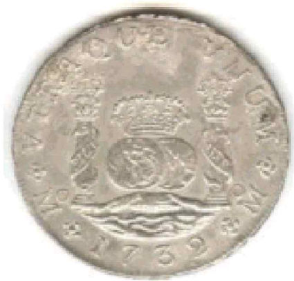
Figure 5 Example of a highly authentic looking but fake columnario which passes all standard numismatic tests but fails contact angle examination.
