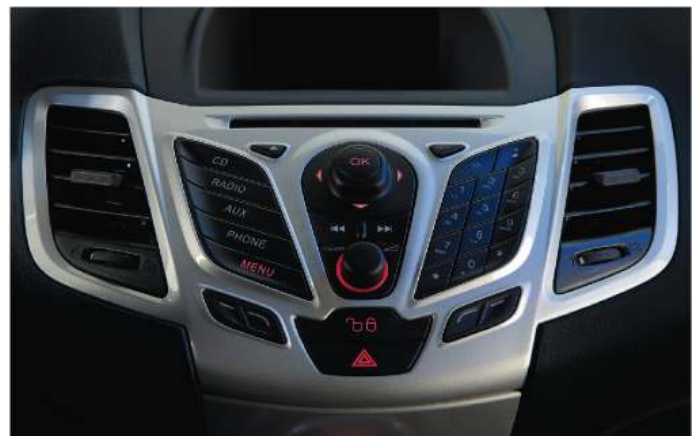
Figure 3 Typical automotive dashboard panel with buttons and switches that must endure many years of poking and handling by both clean and dirty fingers without significant loss of surface finish or imprint readability. (Photo courtesy of Plasmatrete GmbH)
