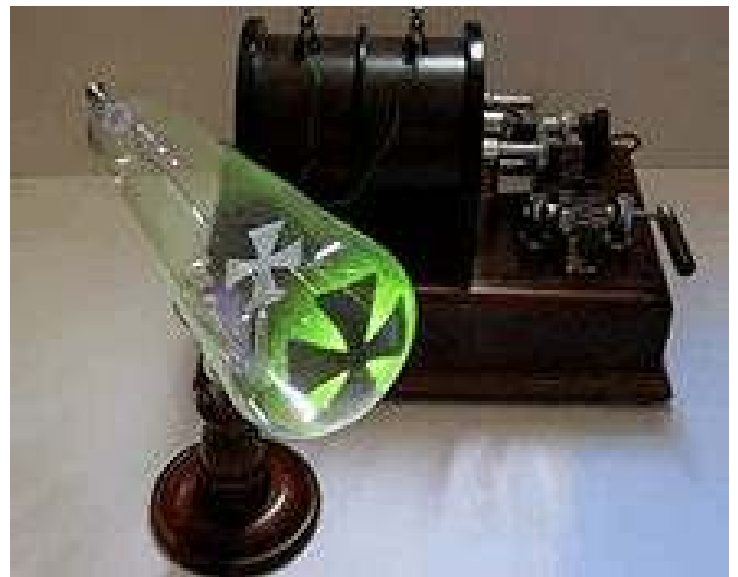
Figure 2 Typical Crooks tube showing fluorescent pattern at end of tube caused by impact of electrons on the glass surface. The sharp outline of the obstructing object indicated that something was traveling in a straight line from the cathode to the anode which were initially called cathode rays.
