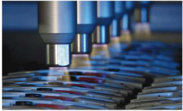
Figure 4 Row of 6 rotary plasma jet nozzles capable of surface treating up to 180,000 small plastic knobs and switches per week. (Photo courtesy Plasmatreat)
